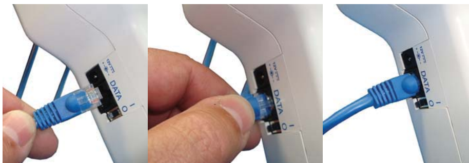
Figure 3-13 Connecting RJ-45 data communications cable
