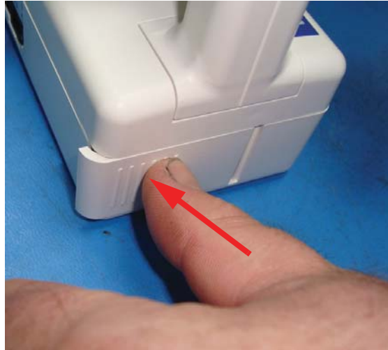
Figure 3-5 Close the Battery Compartment door
