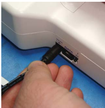
Figure 3-8 Inserting DC power plug.
