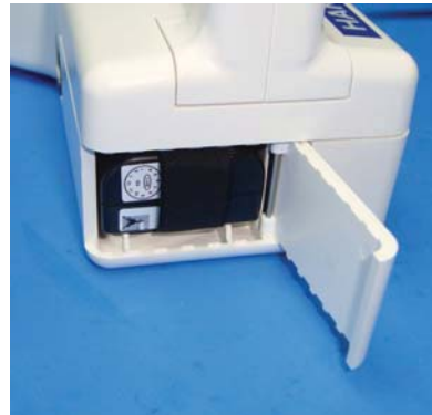
Figure 3-4 Tuck battery release ribbon
