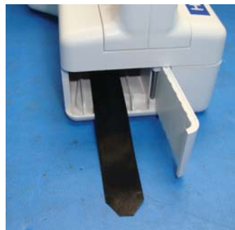
Figure 3-2 Pull Battery release ribbon out
