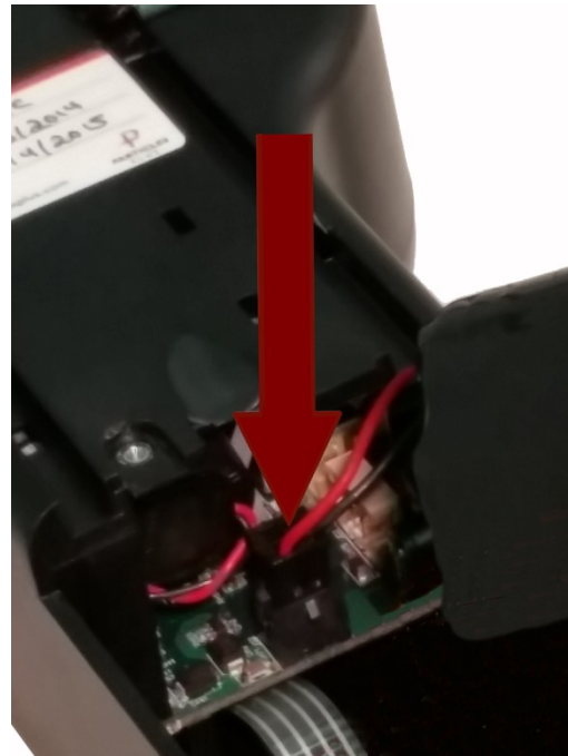
Step 4 – Insert battery connector plug into matching socket on PCB board in battery compartment. NOTE: red and black lead should be on bottom edge of connector.
