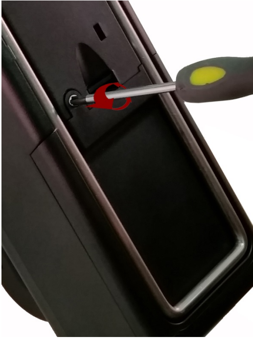
Step 1 - Remove security screw with Phillips screwdriver.
