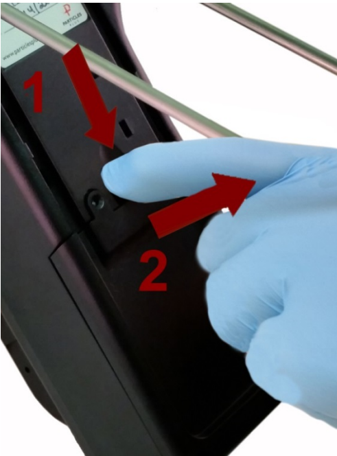
Step 3 – Push down latch while pulling battery compartment cover out and away.
