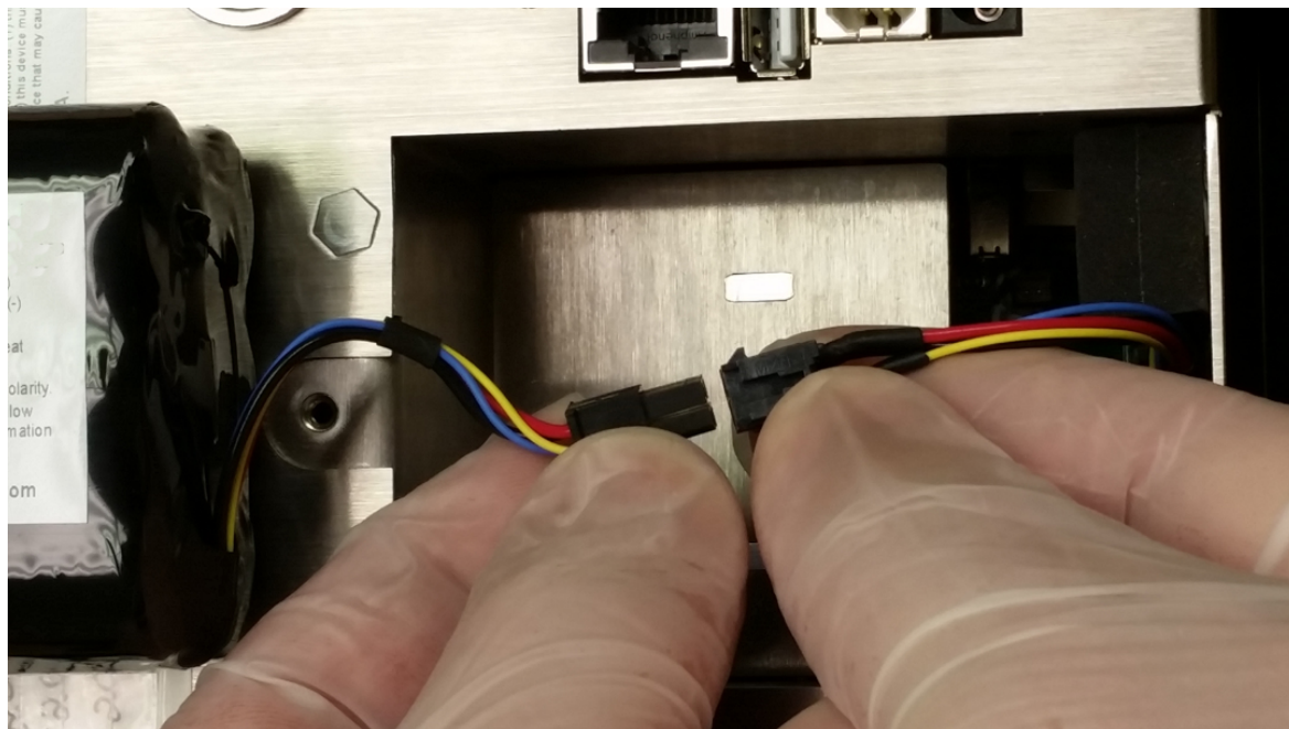
Step 3 – Insert battery connector plug into matching socket on matching wired connector in the battery compartment. NOTE: leads line up color for color and socket has a keyed fit. Carefully tuck the wires neatly back in to the recess in the rear of the battery compartment.
