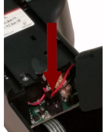
Step 4 – Insert battery connector plug into socket on PCB board in battery compartment. Note: Red and black lead are closest to the bottom edge of the connector.
