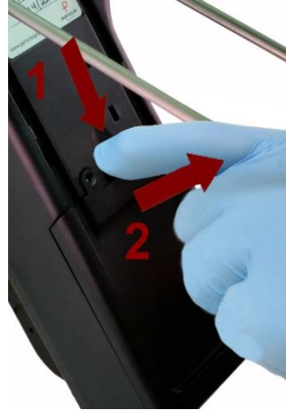
Step 3 – Push down latch while pulling battery compartment cover out and away
