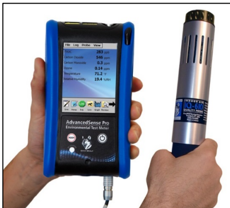
GrayWolf AdvancedSense® PRO meter and DirectSense® probe with installed CO 2 and TVOC (+ 4 optional) sensors.
