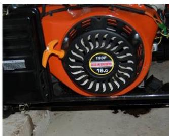
>10,000ppb concentrations are identified near a portable generator, where it’s quickly recognized that a gasoline leak in the back, but hidden by clutter, has dripped, and pooled into a gap along the foundation. Although the high levels in the garage were not above worker exposure levels<sup>G</sup> for gasoline, this was
